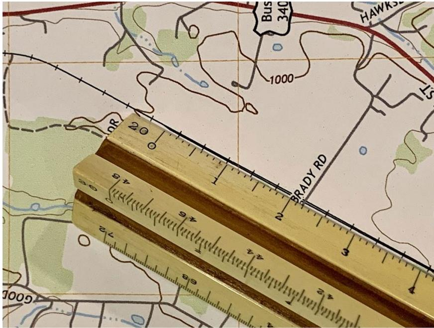
Use the edge of a piece of paper (test score sheet for example) and mark the two points. Use map scale bar for feet located in the bottom center of the map to determine distance between marks to nearest 200-feet.
