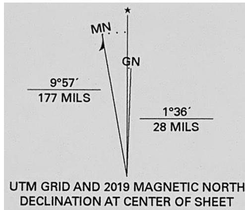
Adjusting values in a clockwise direction require addition of departure values. Adjustments in a counter-clockwise direction subtraction. For the Big Meadows VA quad MN is separated from GN by  $9^{\circ} 57'$  to convert to TN plus  $1^{\circ} 36'$  to convert TN to GN for a total positive difference of  $11^{\circ} 33'$ , round off to  $12^{\circ}$ . Therefore,  $320^{\circ} + 12^{\circ} = 332^{\circ}$
