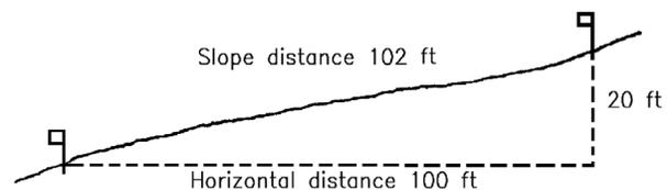
Figure 4. Estimating horizontal distance on a 20 percent slope.
