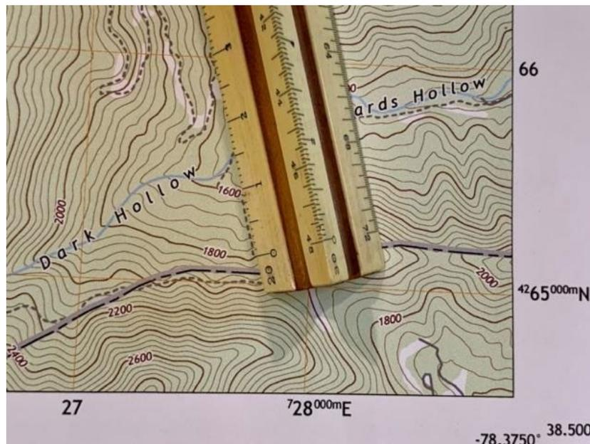
For the trail section in UTM 2765 located between index contour lines 1800 and 1600. The difference in elevation is 200-ft and the distance between the index contours is  $900^+$ -ft. Since the map scale is in 200-foot increments use 1000-feet for the distance. % slope =  $(200 \div 1000) * 100 = 20\%$
